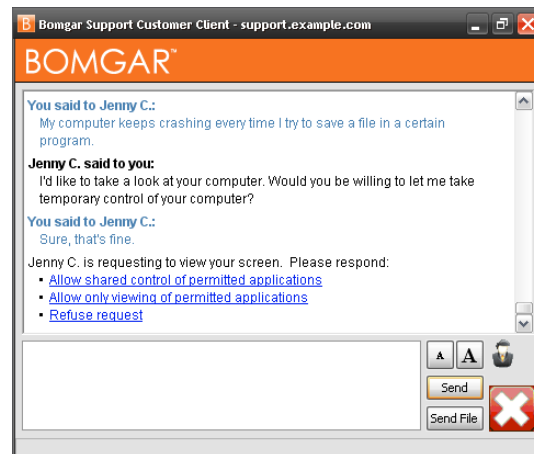
Fig. 4: The customer can chat with the rep, select which applications to share and send files within the customer client interface.
